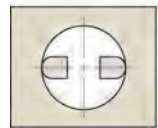
Rounded outside measuring surfaces for measuring inside dimensions
